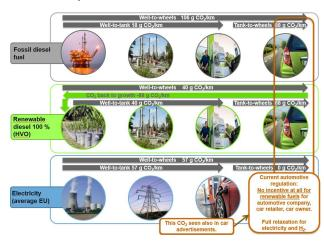
**Well-to-wheels** regulation, even though **ideal**, **is not feasible** for vehicle companies since they can not control  $CO_2$  of fuel and energy production. Case for a biofuel from vegetable oil and average EU electricity. **Biofuel** can be **better than electricity**.
