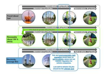
Well-to-wheels case for renewable diesel fuel from waste and average electricity in Finland. Renewable fuels offer remarkable cost-effective solutions to reduce greenhouse gases with minimal investments in vehicle technology and fuel logistics.
