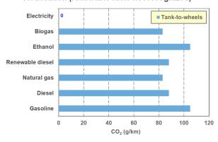
**Well-to-wheels** should be the **ultimate goal** since  $CO_2$  from fuel and energy production and vehicles will be a sum in the atmosphere.  $CO_2$  from fuel and energy production i.e. **well-to-tank shall not be forgotten** when targeting to low greenhouse gas effects.
