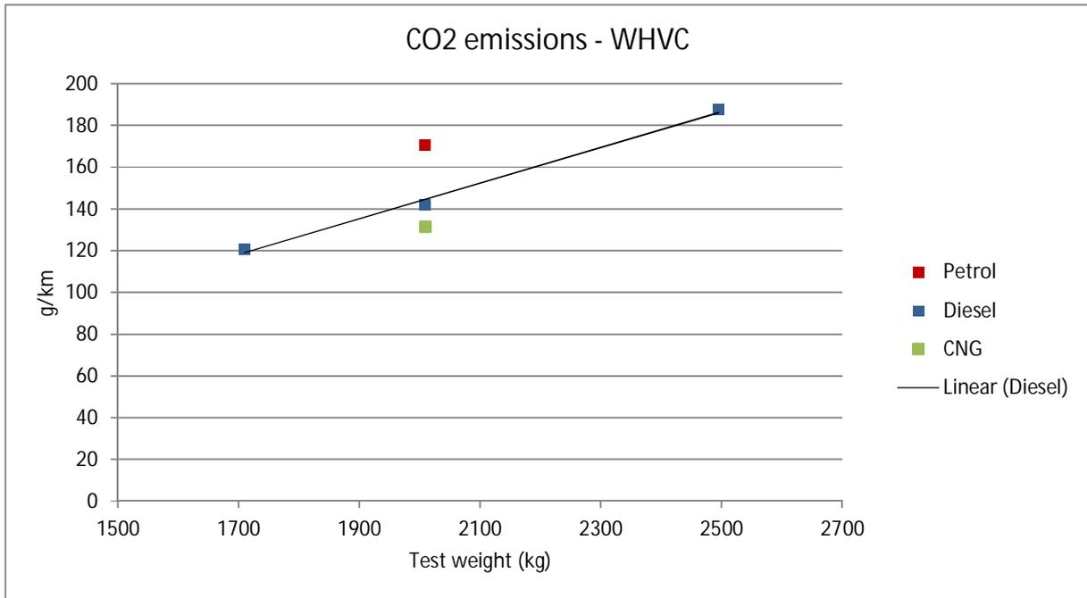
Figure 7.28. CO<sub>2</sub> emission vs. test weight. CH<sub>4</sub> is taken into account for CNG (CO<sub>2eqv</sub>). Category 1 vehicles (vans).
