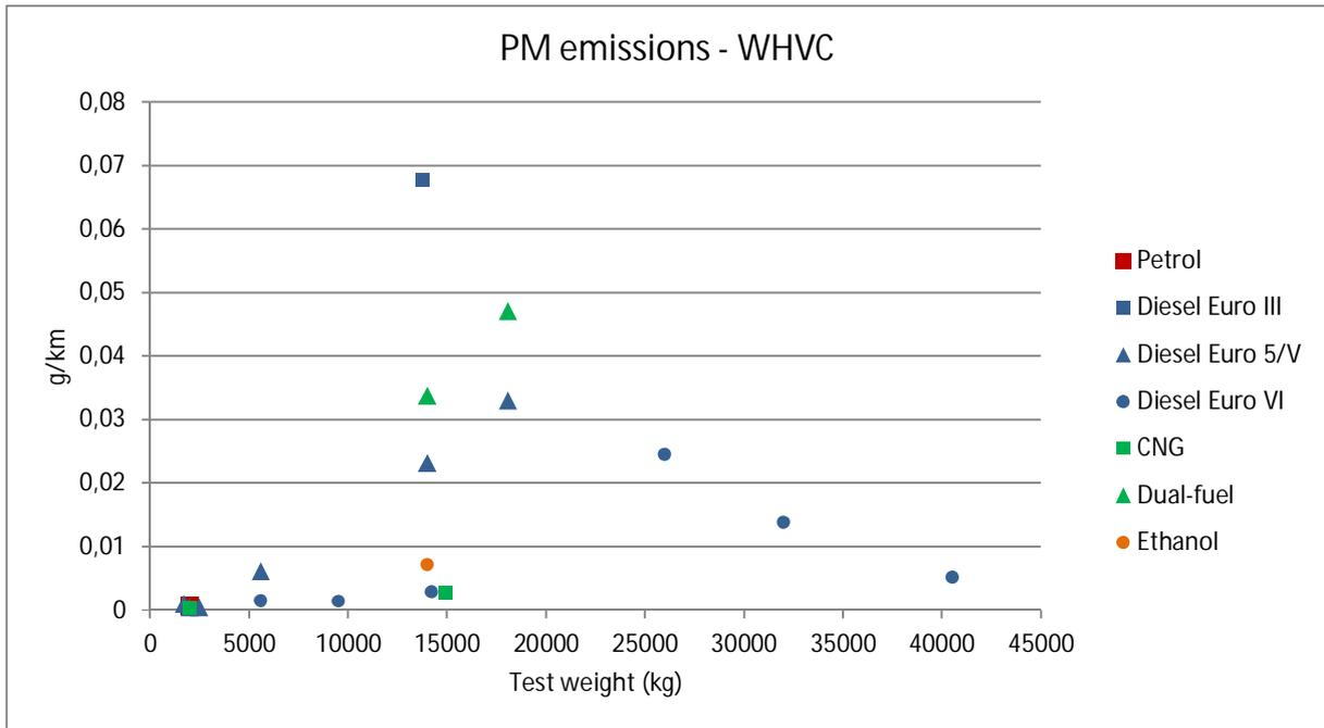
Figure 7.26. PM emissions vs. test weight.
