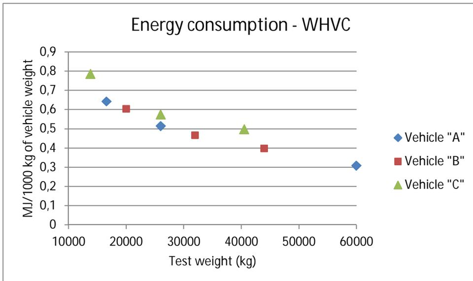
Figure 7.33. Effect of test weight on energy consumption. Euro VI certified Category 3 vehicles. Results presented as MJ per ton of vehicle weight.
