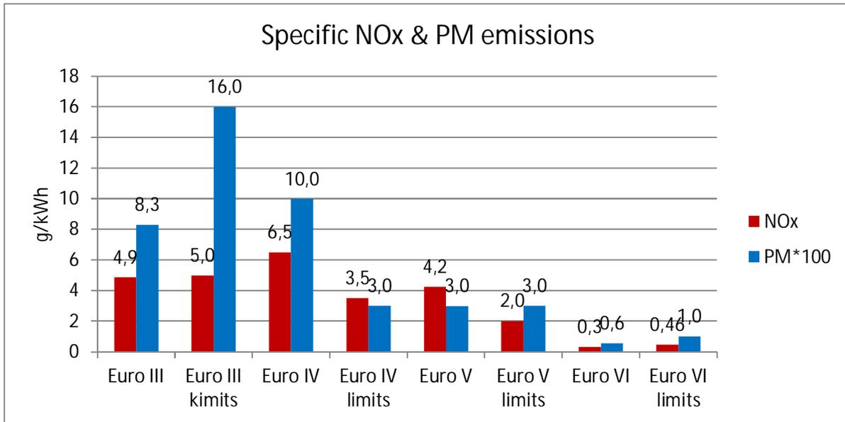
Figure 7.55. Specific NO<sub>x</sub> and PM emissions in g/kWh. Emissions estimated relative to work on the engine crankshaft.
