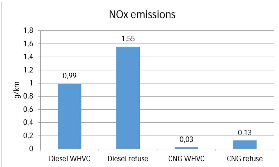
Figure 7.20. NO<sub>x</sub> emissions for two test cycles.
