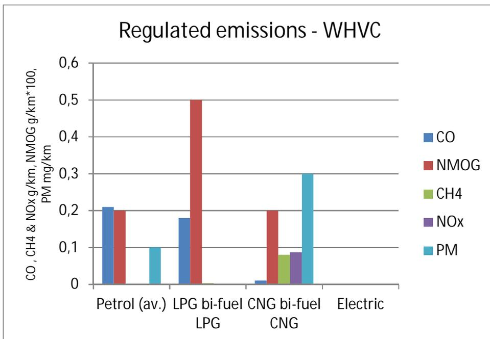
Figure 7.4. Regulated gaseous emissions, Category 1 vans. PM not measured for LPG.
