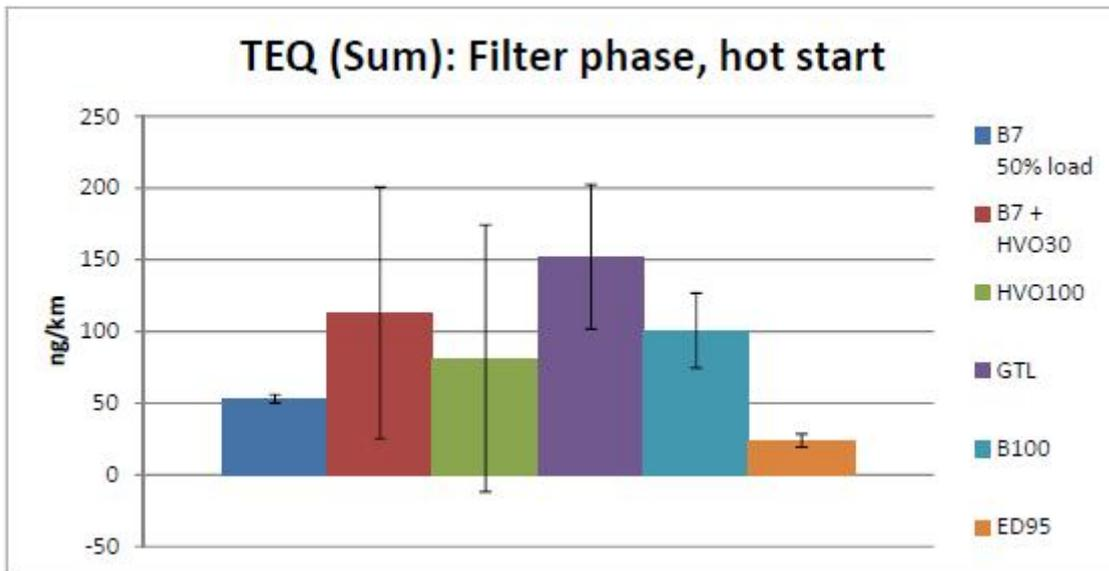
Figure 8.10. Sum of TEQ for filter phase, average of hot start tests.
