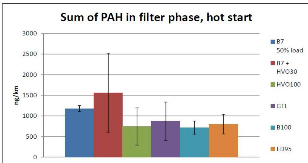
Figure 8.8. Total emissions of analysed PAH in filter phase, averaged results from the hot start tests.
