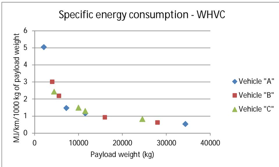
Figure 7.37. The effect of load on specific energy consumption (MJ/1000 kg of payload) for Category 3 vehicles.
