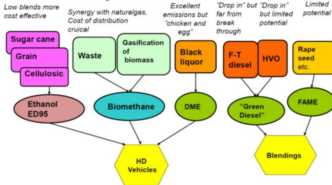
Figure 1.5. Biofuels substituting diesel fuel. (Hådeli 2012)
