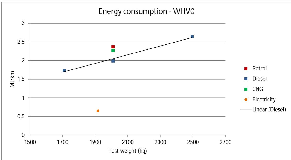
Figure 7.27. Energy consumption vs. test weight. Category 1 vehicles (vans).
