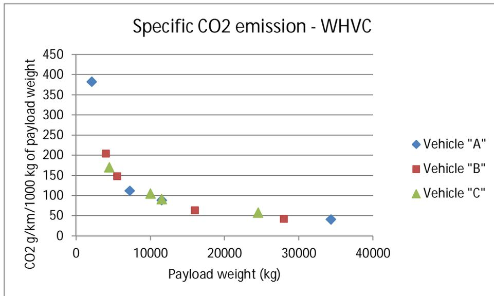
Figure 7.38. The effect of load on specific CO<sub>2</sub> emission (g of CO<sub>2</sub>/1000 kg of payload) for Category 3 vehicles.
