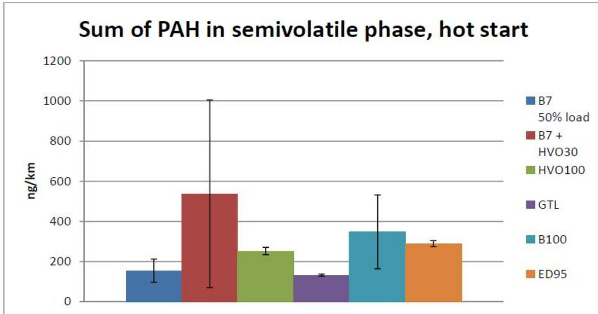
Figure 8.9. Total emissions of analysed PAH in semivolatile phase, averaged results from the hot start tests.
