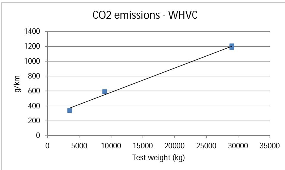
Figure 7.16. CO<sub>2</sub> emission vs. test weight.
