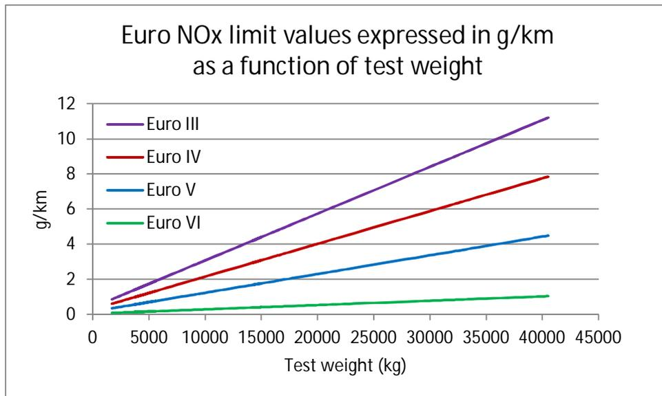
Figure 7.44. Euro III – VI NO<sub>x</sub> limit values expressed in g/km as a function of test weight. No NTE-factors. The Figure should be considered indicative.
