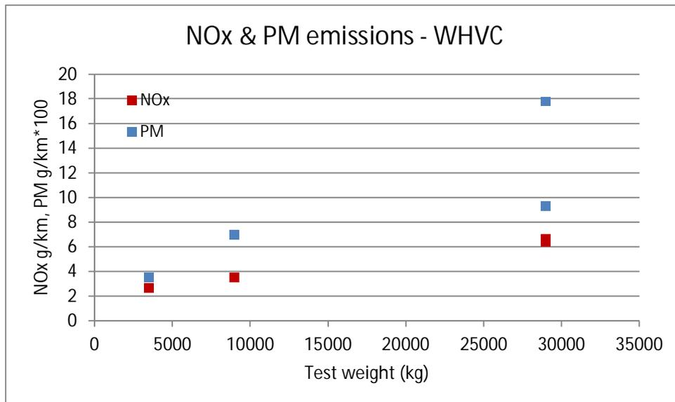
Figure 7.17. NO<sub>x</sub> and PM emissions vs. test weight.
