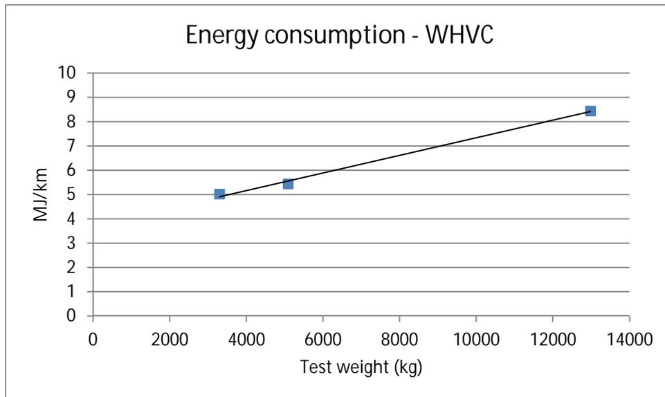
Figure 7.12. Energy consumption vs. test weight.
