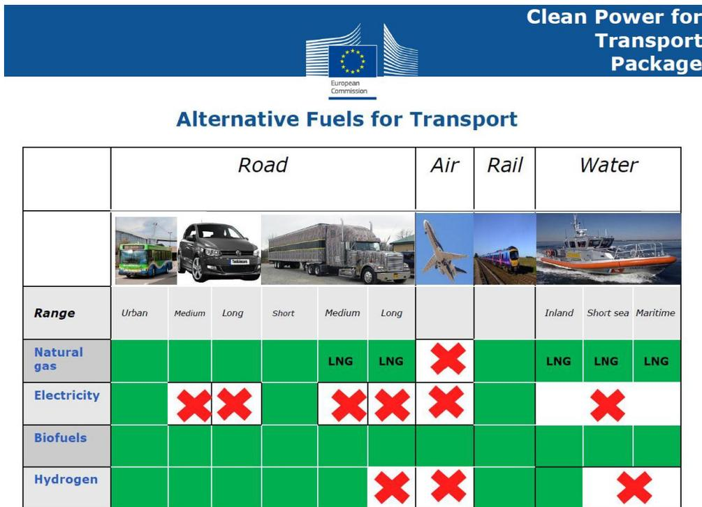
Figure 1.4. Alternative fuels for transport. (Steen 2014)
