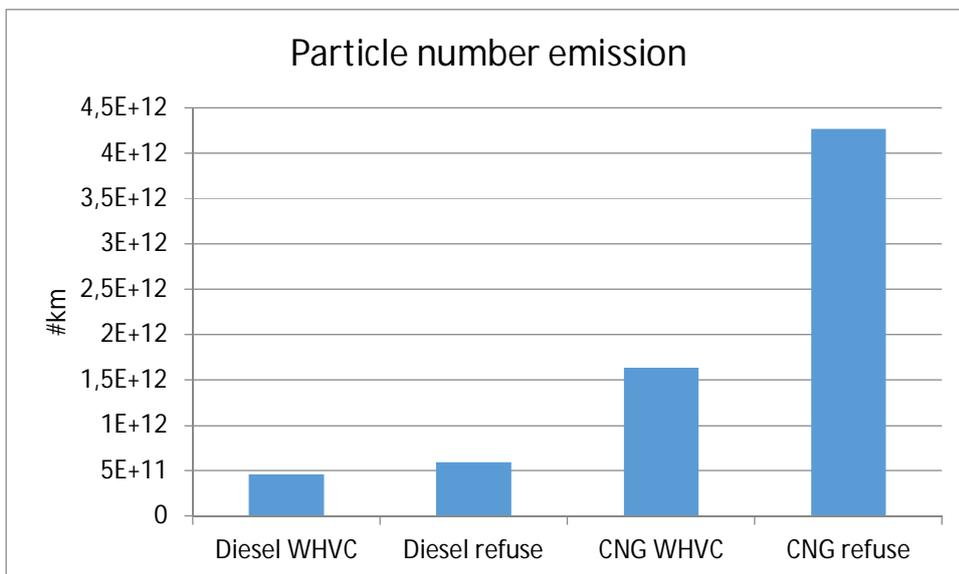
Figure 7.21. Particulate number emissions for two test cycles.
