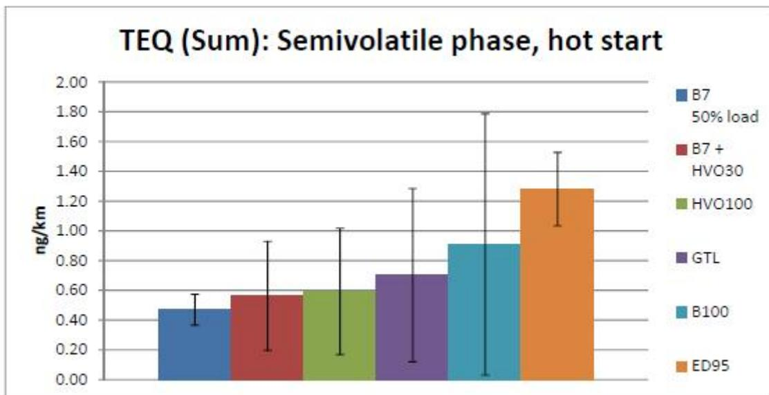
Figure 8.11. Sum of TEQ for semivolatile phase, average of hot start tests.
