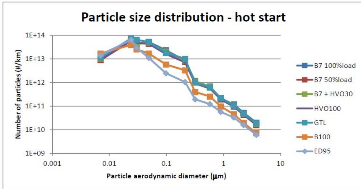
Figure 8.7. Particle number emissions – averaged results from hot start tests.
