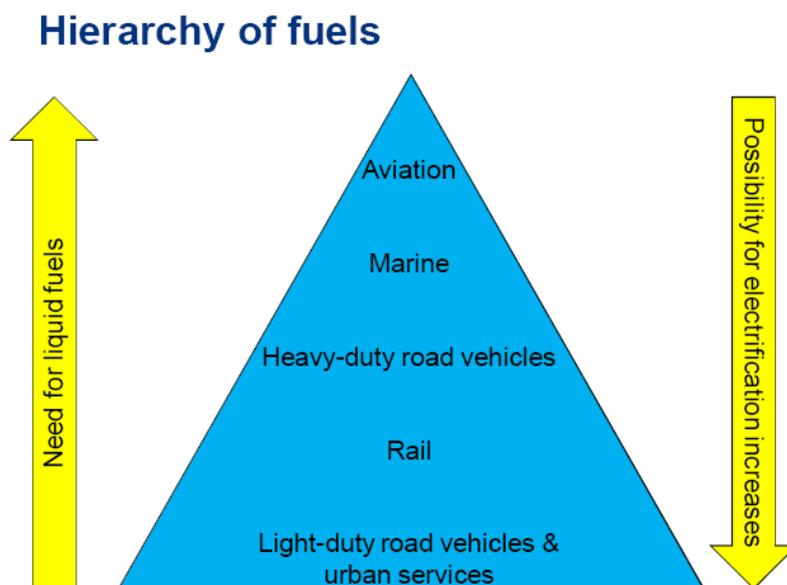
Figure 1.3. Hierarchy of fuels. Based on (Alternative propulsion for the transport of the future 2013).
