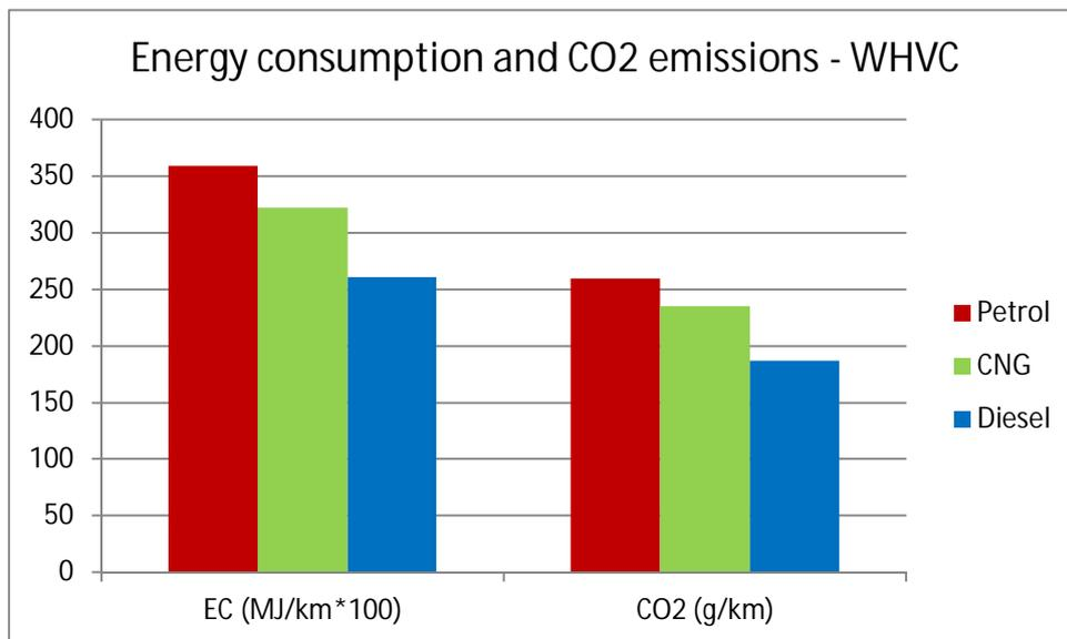
Figure 7.41. Energy consumption and CO<sub>2</sub> emissions. Euro 4 certified Category 1 pick-ups. CH<sub>4</sub> is taken into account for CNG (CO<sub>2eqv</sub>).
