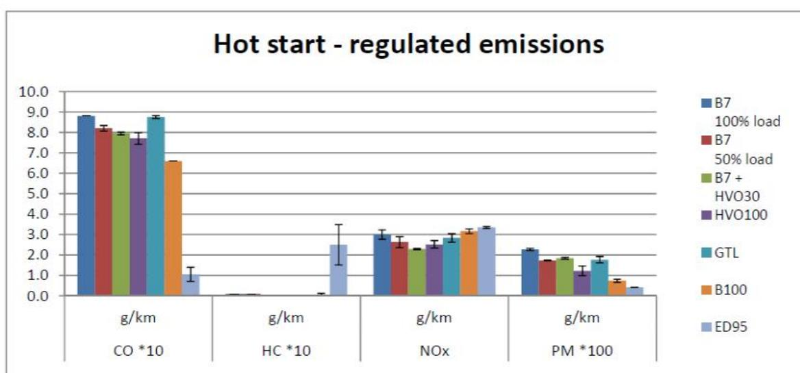
Figure 8.4. Regulated emissions from hot start tests, averaged from two tests.
