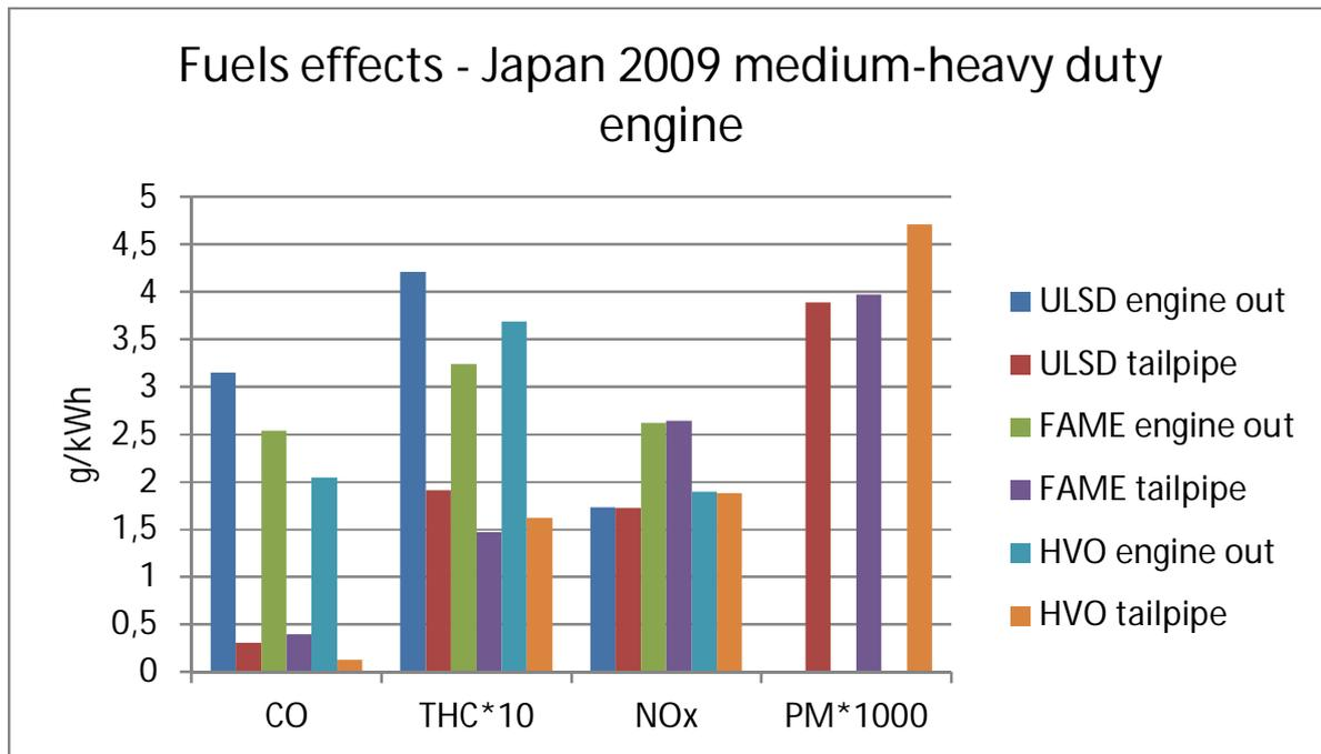
Figure 8.3. Fuel effects on regulated emissions of a Japan 2009 certified medium heavy-duty truck engine.
