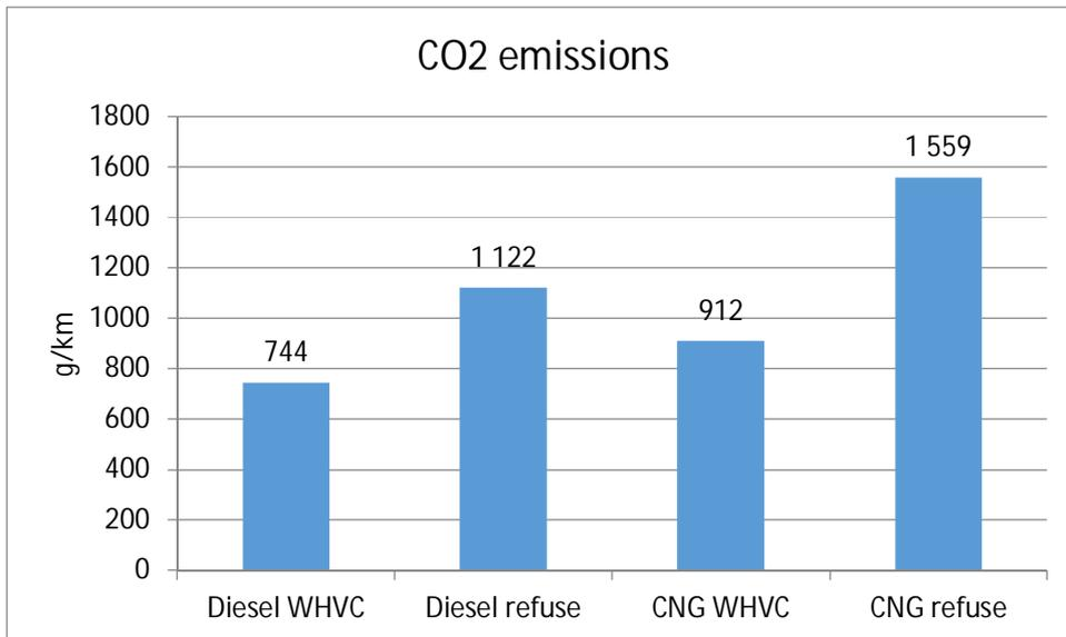
Figure 7.19. CO<sub>2</sub> emission for two test cycles. CH<sub>4</sub> is taken into account for CNG (CO<sub>2</sub><sub>eqv</sub>).
