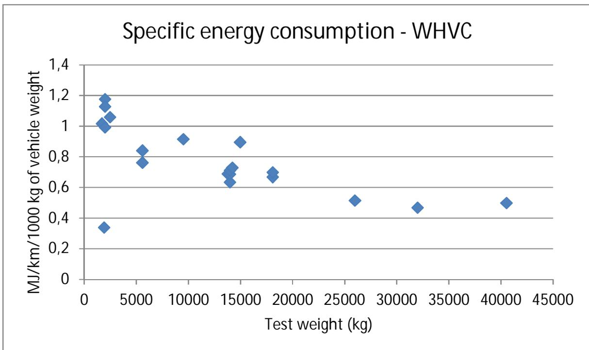
Figure 7.23. Energy consumption vs. test weight.
