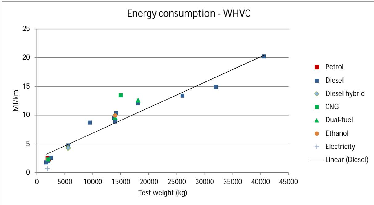
Figure 7.22. Energy consumption vs. test weight.
