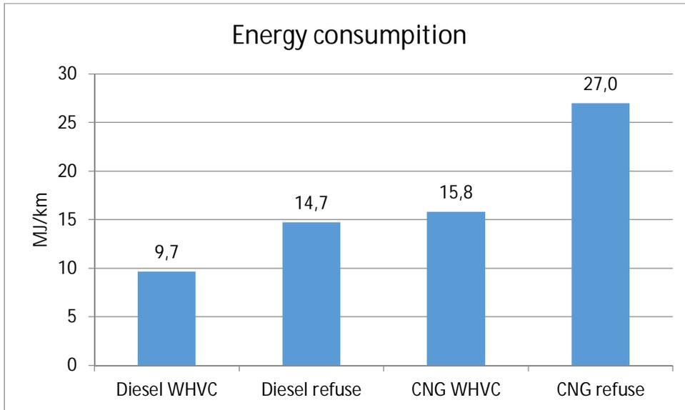
Figure 7.18. Energy consumption for two test cycles.
