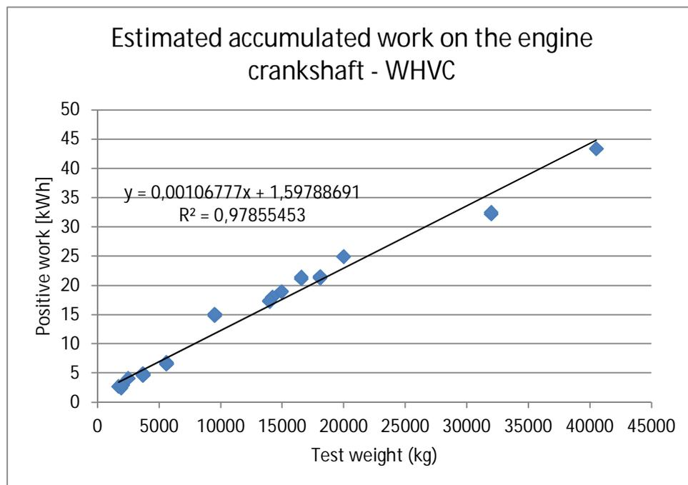
Figure 7.43. Estimated accumulated work on the engine crankshaft in the WHVC test cycle as a function of test mass. Powertrain and auxiliary losses estimated at a total of 20 %.
