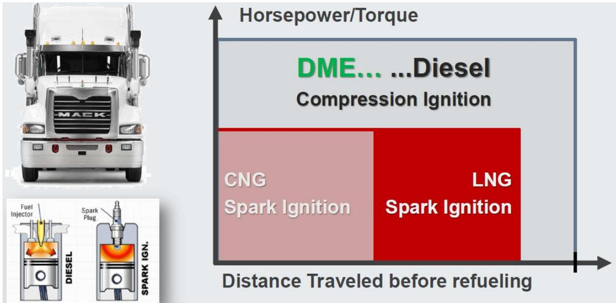
Figure 1.6. DME performance vs. spark-ignited CNG and LNG. (Alt 2014)
