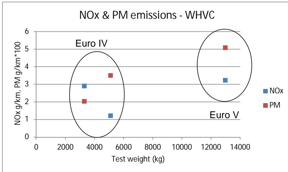
Figure 7.14. NO<sub>x</sub> and PM emissions vs. test weight.
