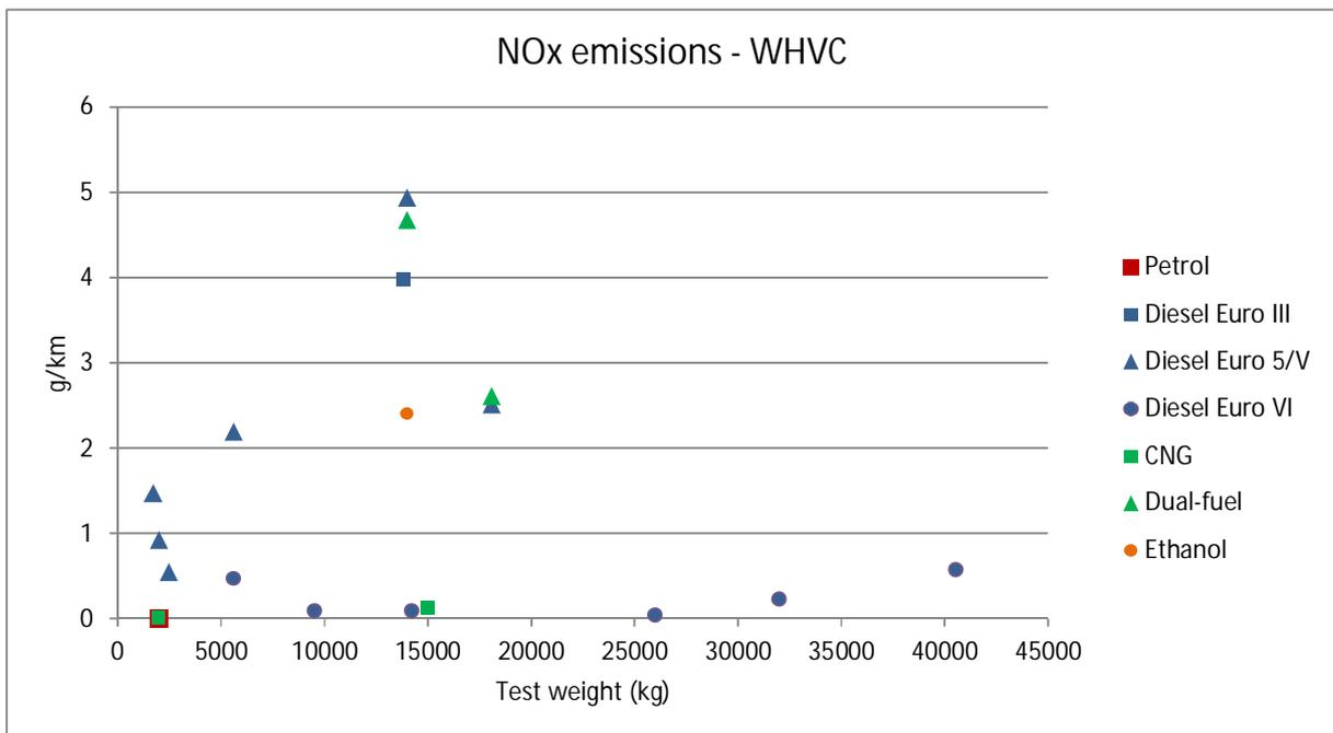
Figure 7.25. NO<sub>x</sub> emissions vs. test weight.
