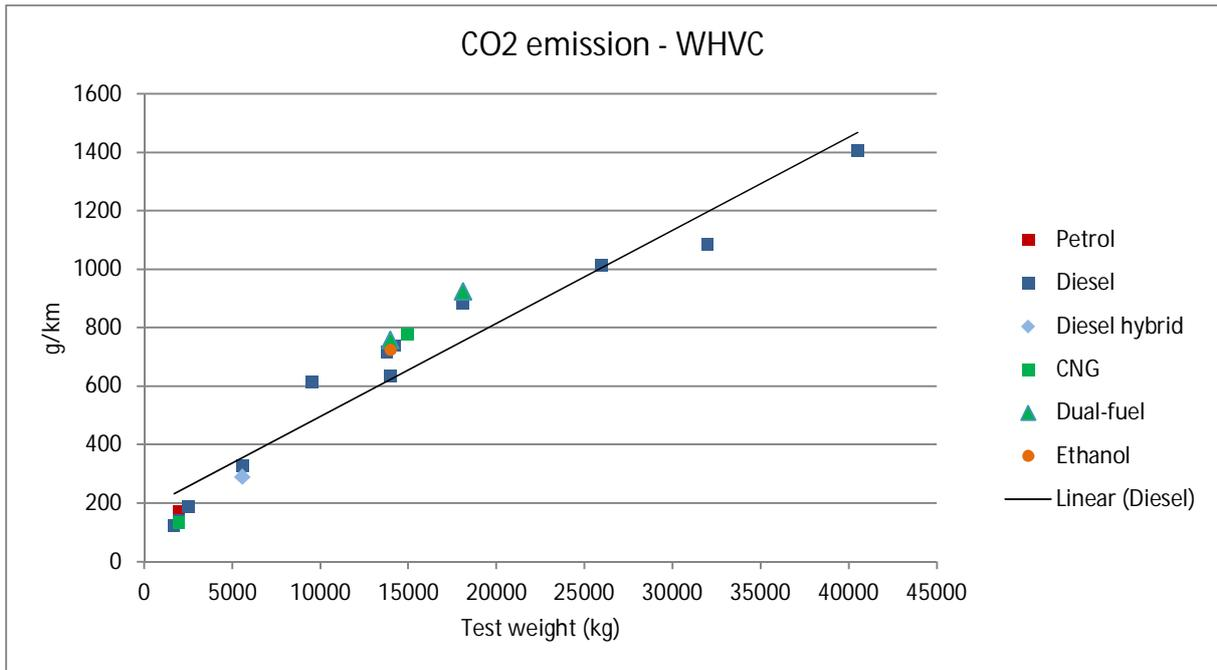
Figure 7.24. CO<sub>2</sub> emission vs. test weight. CH<sub>4</sub> is taken into account for CNG (CO<sub>2</sub><sub>eqv</sub>).
